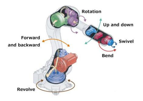
$\rightarrow$  Basic parts and movements of an industrial robot
